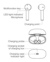
Multi-function button LED light indicator Microphone Charging point In and out case indicator Charging probe Charging socket of charging box Charging case indicator light
